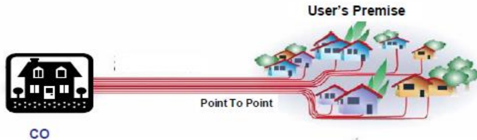
Fig : 4 Home Run Fiber (Point-to-Point) architecture
